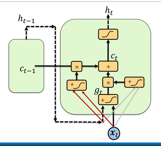
Forget gate Controls how past internal state  $c_{t-1}$ contributes to  $c_t$
