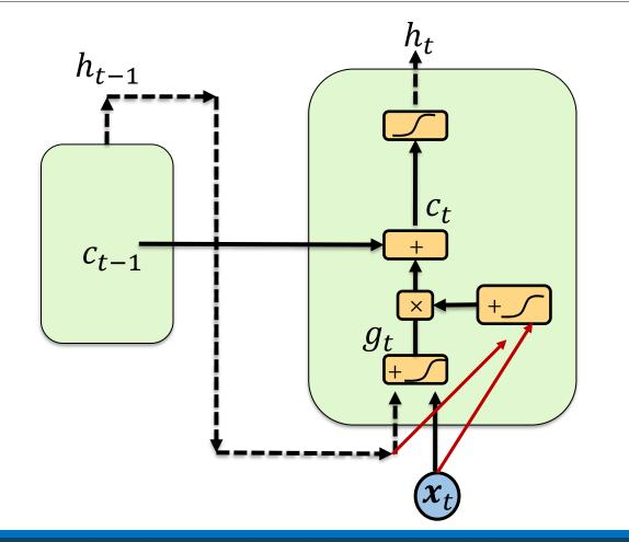
Input gate Controls how inputs contribute to the internal state
