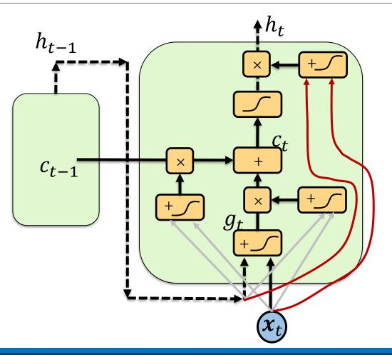
Output gate Controls what part of the internal state is propagated out of the cell
