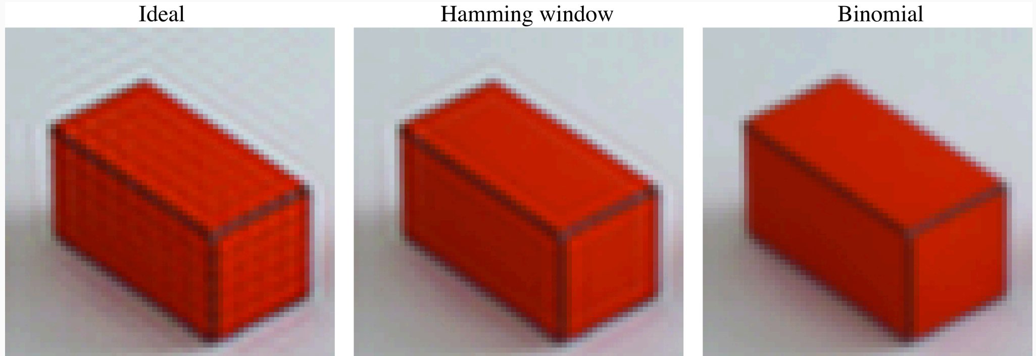
Figure 9: note the ringing artifacts with the ideal filter. Source: visionbook
