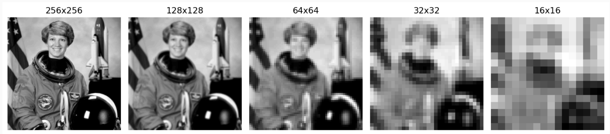
Figure 17: Gaussian pyramid: each level is blurred and downsampled by 2 from the previous Coarse levels highlight global features, useful for object detection, which requires also global-scale features.
