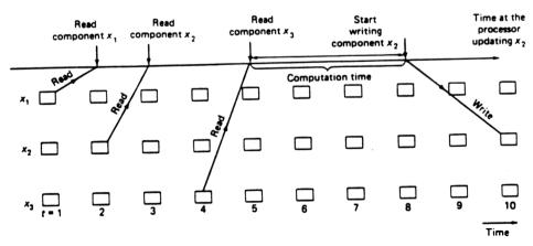
Fig. 7. Illustration of a component update in a shared memory multiprocessor. Here  $x_2$  is viewed as being updated at time t = 9 ( $9 \in T^2$ ), with  $\tau_1^2(9) = 1$ ,  $\tau_2^2(9) = 2$ , and  $\tau_4^2(9) = 4$ . The updated value of  $x_2$  is entered at the corresponding register at t = 10. Several components can be simultaneously in the process of being updated, and the values of  $\tau_1^i(t)$  can be unpredictable.
