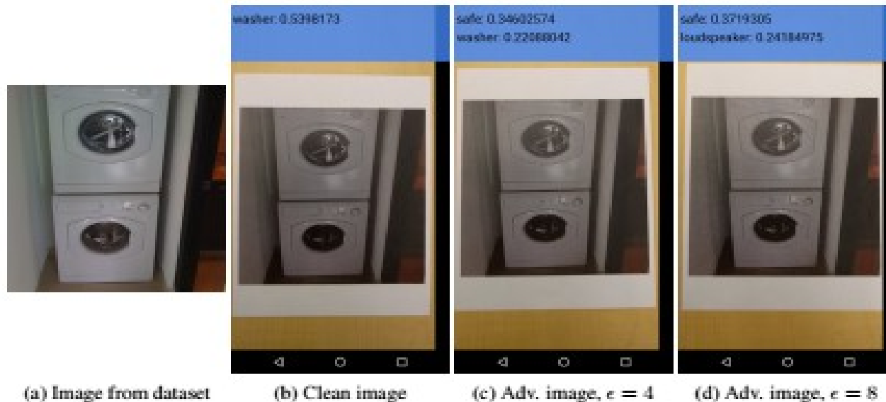
Figure 1: Demonstration of a black box attack (in which the attack is constructed without access to the model) on a phone app for image classification using physical adversarial examples. We took a clean image from the dataset (a) and used it to generate adversarial images with various sizes of adversarial perturbation \epsilon . Then we printed clean and adversarial images and used the TensorFlow Camera Demo app to classify them. A clean image (b) is recognized correctly as a “washer” when perceived through the camera, while adversarial images (c) and (d) are misclassified. See video of full demo at https://youtu.be/zQ_uMenoBCk .
