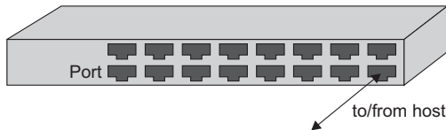
Figure 8.2: A 16-port switch as used in local-area networks.
