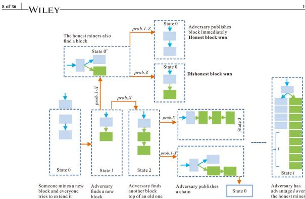
FIGURE 3 State machine a selfish attack
